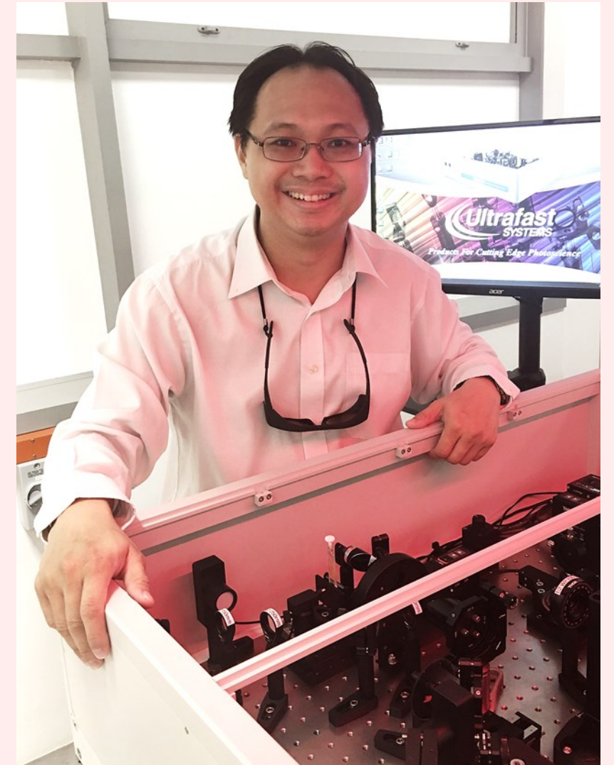
Associate Professor Sum Tze Chien with spectrometers used to track the hot carrier cooling processes in perovskite nanocrystals. Photo: NTU
